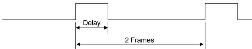
If the unit is not synchronising, such as loss of I/P or Freeze, then the delay output is blanked (static low). It is expected under these conditions that the audio processing will hold its current delay from the last valid measurement until a pulse re-appears.
