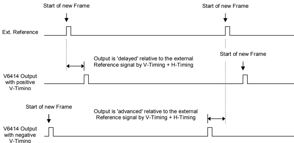
This drawing illustrates the **Reference-to-Output** timing relationship when operating a V6414 in its Frame-Synchroniser mode.
