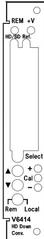
The front panel is similar to other complex V1600 types. It provides the user with total control and monitoring of the unit without the need to consult manuals and read unlabelled indicators.
