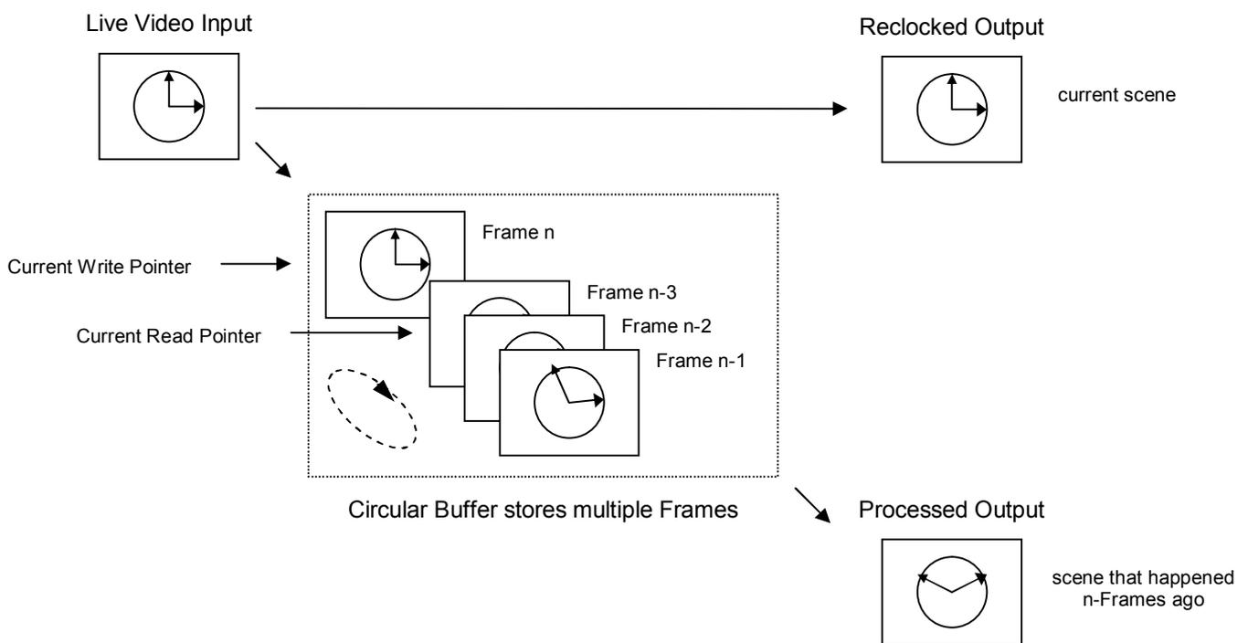
Live Video data gets written into a circular buffer (Frame-Store), which is  $n+1$  frames deep ( $n$  is the number of frames the output gets delayed on top of the variable delay). The buffer's write-pointer lags exactly one frame behind the buffer's read pointer, which means that a frame that got written  $n$ -frames ago, will be read one frame prior to it gets overwritten by a new frame.
